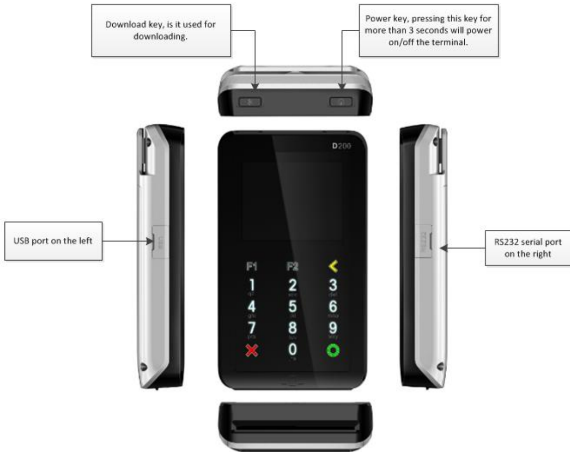
Figure 2-1 D200 appearance and its ports
