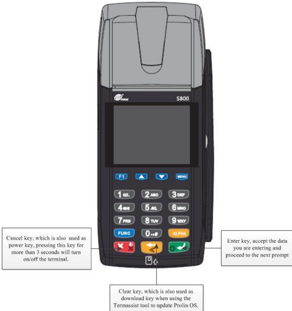
Figure 2-2 Appearance and key descriptions of S800
